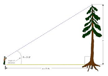
The path to the base of the object plus the path to the top of the object plus the height of the object forms a right triangle. By knowing the distance to the base and the angle, we can apply some basic trigonometry to determine the height of the object. In this activity you will determine the height of objects around the Cove.
